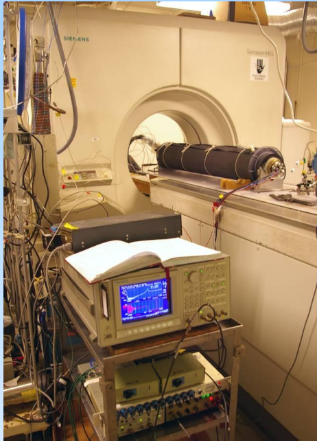
X-ray CT imaging of resonant bar enclosed in thermal jacket
